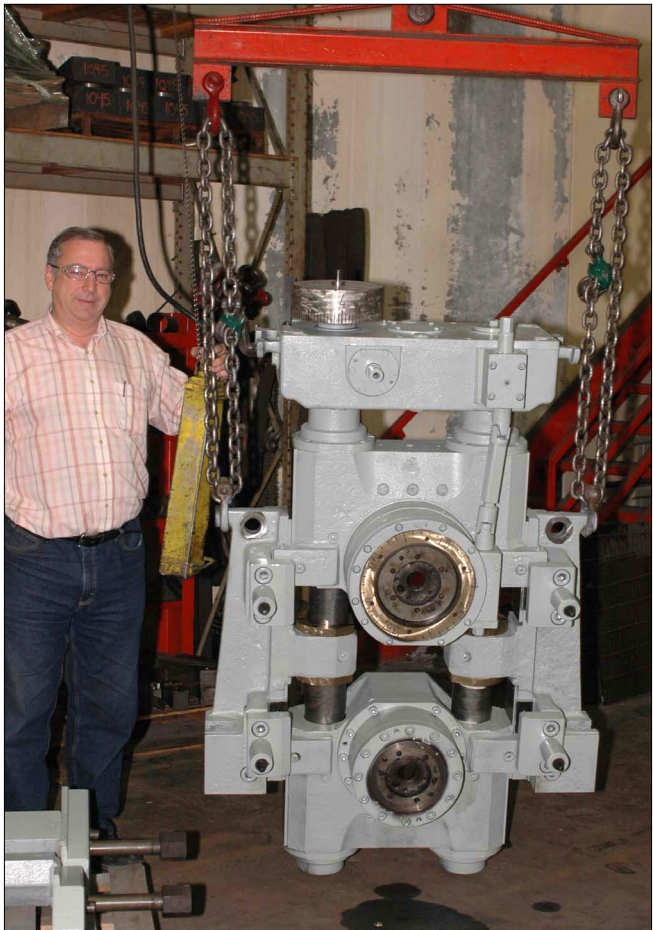
PHOTO BY MARGARET A. ONTL Ken Konrad stands by a rolling mill stand, one of the pieces of equipment they repair and restore for the steel mill industry.
