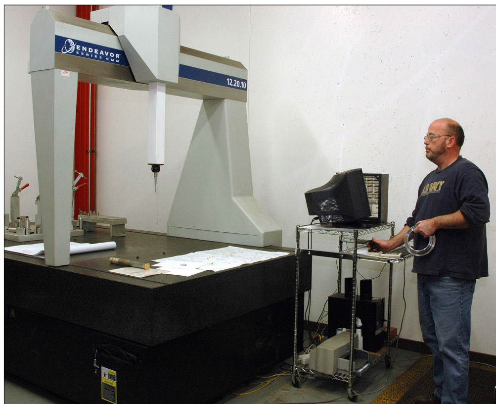
Tim Johnson, who has worked for the Konrads for 24 years is the quality control manager. He is demonstrating the Coordinate Measuring Machine which uses a ceramic quill to measure pieces before and during production to make sure they match the specifications and tolerances.
