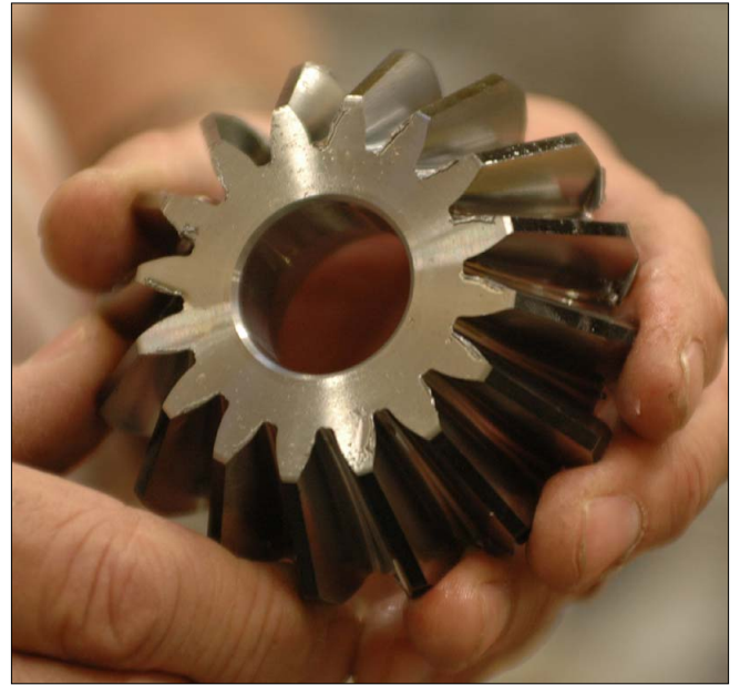
PHOTO BY MARGARET A. ONTL One of the gears manufactured by Konrad, before it is finished and hardened.
