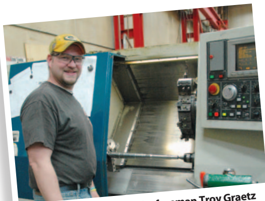
Konrad Marine machinist foreman Troy Graetz performing a prop shaft turning operation.
